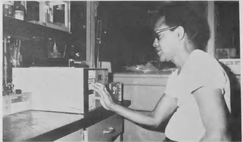
Lab Assistant F. Holmond is running a test through push-button action for sulfur content on the new X-Ray Sulfur Analyzer.
